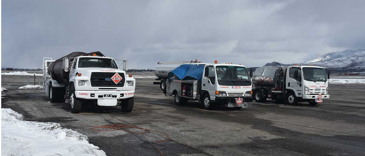
Figure 15: Three of the five Leading Edge fuel trucks. The company covers their trucks with plastic tarps, as shown here. This has never been observed elsewhere and raises questions of the functionality of the trucks and the purity of the fuel they pump.
