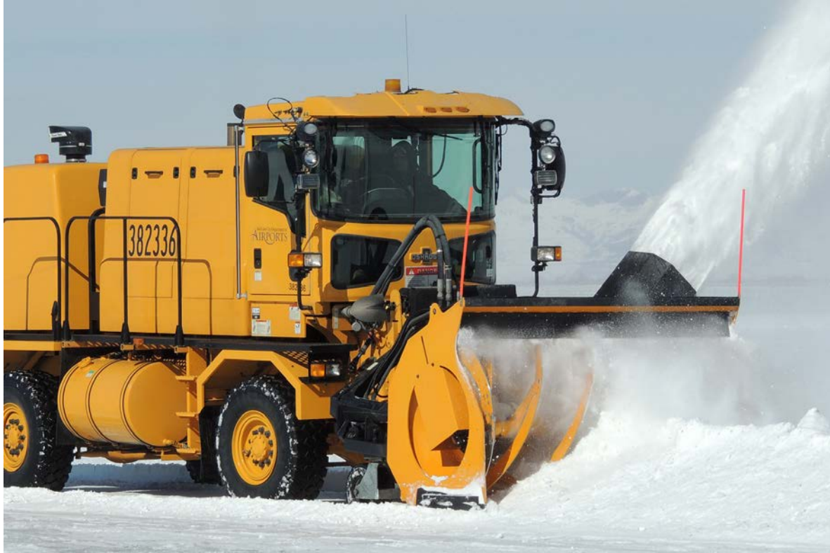
Figure 6: A modern "snow eater" typically found at modern airports. These systems prevent dangerous berms of snow from accumulating at the edges of runways.
