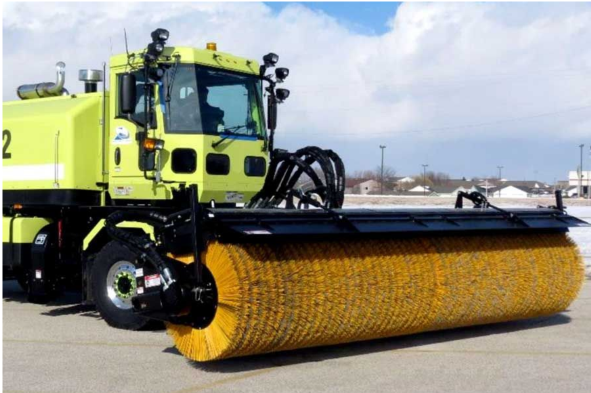
Figure 5: An example of a modern snow “broom” used to completely remove light snow from runways.
