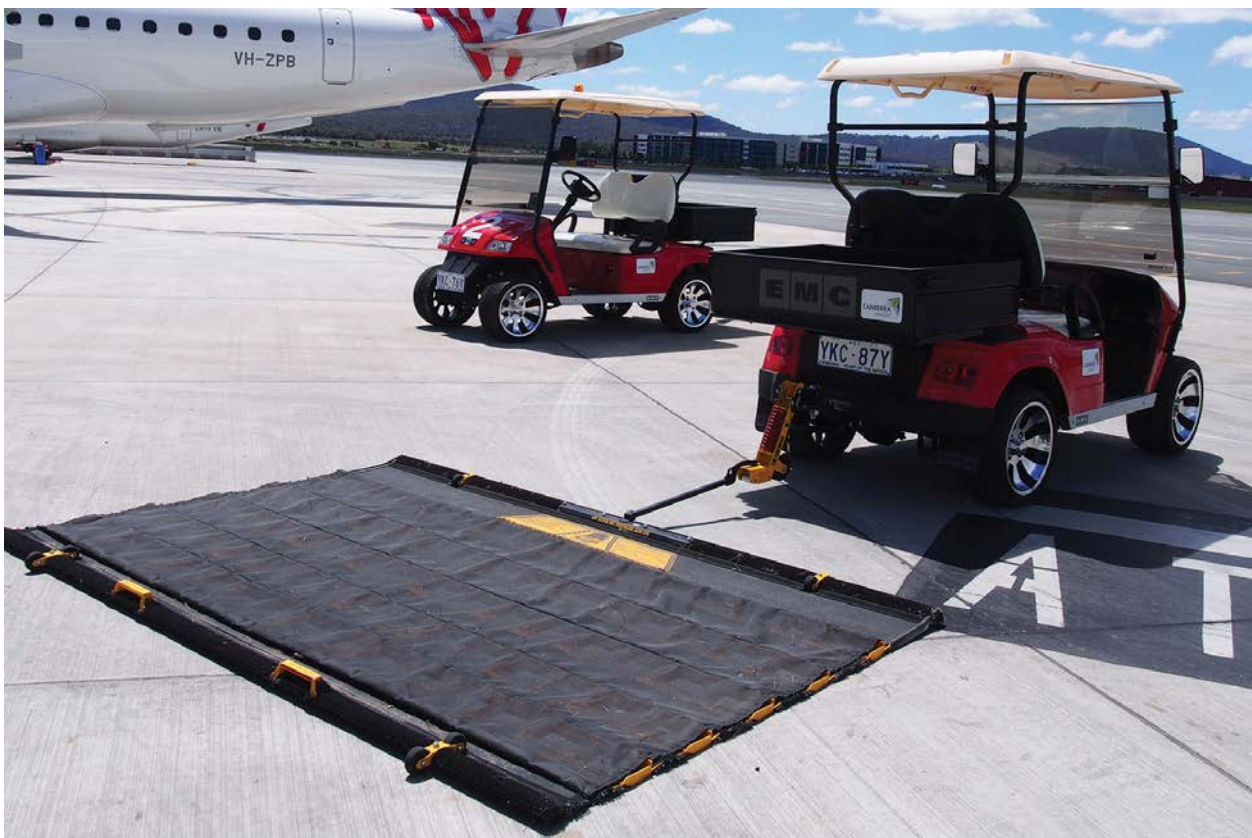
Figure 25 introduces an inexpensive tool which can eliminate FOD. This is called a "FODBuster."
